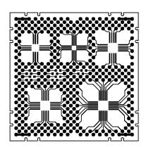
Supports 16 & 28 Pins with a .5mm pitch, 20 Pin with a .65mm pitch and 12 & 16 Pins with a .8mm pitch for QFN devices
