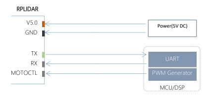
Figure 3-3 RPLIDAR A3 Pins Reference Design
