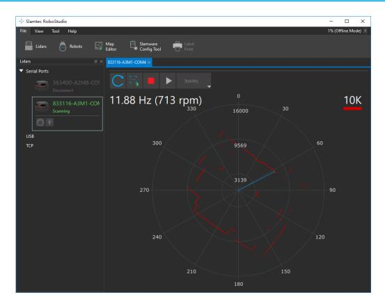
Figure 2-9 The Scan Outline by RPLIDAR in RoboStudio
