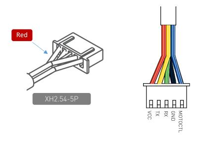
Figure 3-1 RPLIDAR A3 Pins
