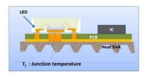
If the thermal dissipation is good enough, the junction temperature will be lower and the lifetime performance will be better.
