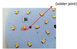
You can use the high-temperature thermal conductivity glue (Such as SatlonD-3/606...etc.) to fix the thermal couple to the solder joint then measure the temperature. Once you got the T<sub>S</sub> temperature measurement data, you can calculate the junction temperature based on the measurement data of the Ts. The details of the calculation method are shown in the following page:
