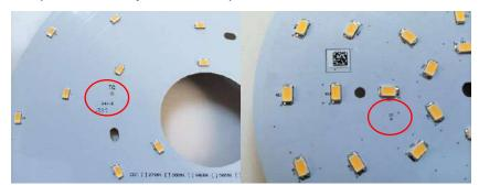
You can use the high-temperature thermal conductivity glue (Such as SatlonD-3/606...etc.) to fix the thermal couple to the  $T_C$  point then measure the temperature. Once you got the T<sub>C</sub> temperature measurement data, you can calculate the junction temperature based on the measurement data of the T<sub>C</sub>. The details of the calculation method are shown in the following page:
