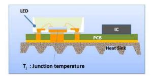
If the thermal dissipation is good enough, the junction temperature will be lower and the lifetime performance will be better.
