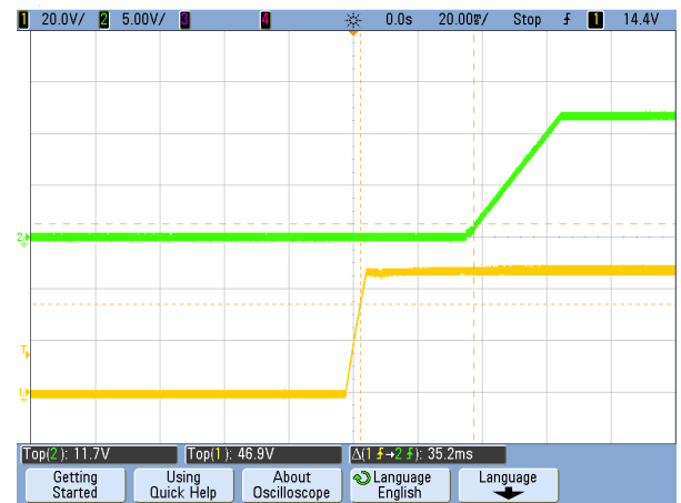
Figure 21. Vin Start-up Delay (CH2: Vout, CH1: Vin) (Vin=48V, Iload=33A, Cload=5500µF, Ta=+25°C, 20mS/div)
