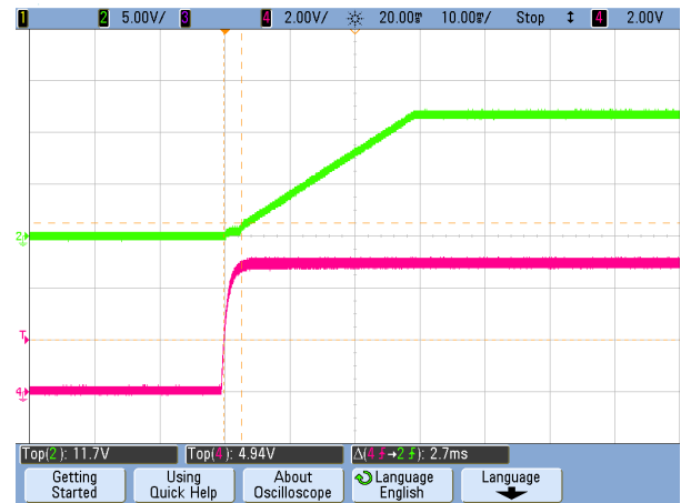
Figure 21. Vin Start-up Delay (CH2: Vout, CH1: Vin) (Vin=48V, Iload=33A, Cload=5500µF, Ta=+25°C, 20mS/div)
