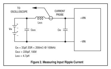
In critical applications, output ripple and noise (also referred to as periodic and random deviations or PARD) may be reduced by adding filter elements such as multiple external capacitors. Be sure to calculate component temperature rise from reflected AC current dissipated inside capacitor ESR.
