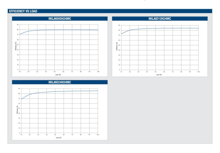
5.7kVDC Isolated 6W Dual Output Gate Drive SM DC-DC Converters
