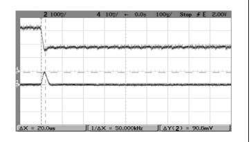
Step Load Transient Response (Vin=24V, Vout=nominal, Cload=0, Iout=0.5A to 1.0A, Slew=1A/ $\mu$ S, Ta=+25°C.) Trace 2=Vout, 100 mV/div. Trace 4=lout, 0.5A/div.
