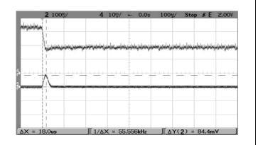
Step Load Transient Response (Vin=12V, Vout=nominal, Cload=0, Iout=0.75A to 1.5A, Slew=1A/ $\mu$ S, Ta=+25°C.) Trace 2=Vout, 100 mV/div. Trace 4=Iout, 0.5A/div.
