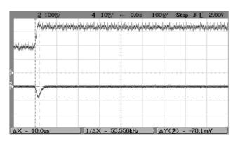
Step Load Transient Response (Vin=12V, Vout=nominal, Cload=0, Iout=1.5A to 0.75A, Slew=1A/µS, Ta=+25°C.) Trace 2=Vout, 100 mV/div. Trace 4=Iout, 0.5A/div.
