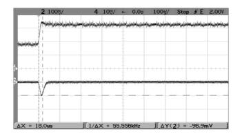
Step Load Transient Response (Vin=15V, Vout=nominal, Cload=0, Iout=1.0A to 0.5A, Slew=1A/µS, Ta=+25°C.) Trace 2=Vout, 100 mV/div. Trace 4=Iout, 0.5A/div.
