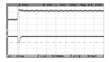
Step Load Transient Response (Vin=7V, Vout=nominal, Cload=0, lout=1.5A to 0.75A, Slew=1A/µS, Ta=+25°C.) Trace 2=Vout, 100 mV/div. Trace 4=lout, 0.5A/div.
