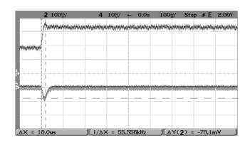
Step Load Transient Response (Vin=36V, Vout=nominal, Cload=0, Iout=1.0A to 0.5A, Slew=1A/ $\mu$ S, Ta=+25°C.) Trace 2=Vout, 100 mV/div. Trace 4=Iout, 0.5A/div.
