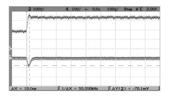
Step Load Transient Response (Vin=36V, Vout=nominal, Cload=0, lout=1.5A to 0.75A, Slew=1A/ $\mu$ S, Ta=+25°C.) Trace 2=Vout, 100 mV/div. Trace 4=lout, 0.5A/div.
