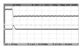
Step Load Transient Response (Vin=36V, Vout=nominal, Cload=0, Iout=0.75A to 1.5A, SIew=1A/µS, Ta=+25°C.) Trace 2=Vout, 100 mV/div. Trace 4=Iout, 0.5A/div.
