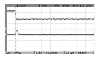
Step Load Transient Response (Vin=36V, Vout=nominal, Cload=0, lout=0.5A to 1.0A, Slew=1A/µS, Ta=+25°C.) Trace 2=Vout, 100 mV/div. Trace 4=lout, 0.5A/div.
