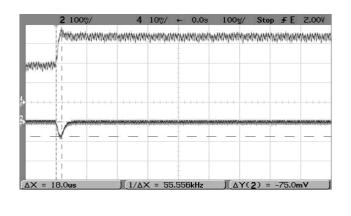
Step Load Transient Response (Vin=36V, Vout=nominal, Cload=0, lout=1.5A to 0.75A, Slew=1A/μS, Ta=+25°C.) Trace 2=Vout, 100 mV/div. Trace 4=lout, 0.5A/div.
