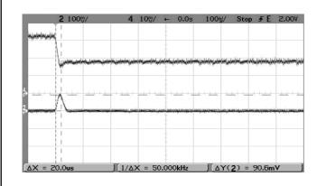
Step Load Transient Response (Vin=12V, Vout=nominal, Cload=0, Iout=0.75A to 1.5A, SIew=1A/ $\mu$ S, Ta=+25°C.) Trace 2=Vout, 100 mV/div. Trace 4=Iout, 0.5A/div.
