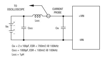
Figure 3 Measuring Input Ripple Current
