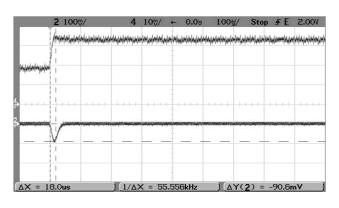
Step Load Transient Response (Vin=24V, Vout=nominal, Cload=0, lout=1.0A to 0.5A, Slew=1A/µS, Ta=+25°C.) Trace 2=Vout, 100 mV/div. Trace 4=lout, 0.5A/div.
