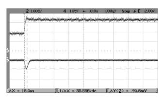
Step Load Transient Response (Vin=12V, Vout=nominal, Cload=0, Iout=1.5A to 0.75A, Slew=1A/µS, Ta=+25°C.) Trace 2=Vout, 100 mV/div. Trace 4=lout, 0.5A/div.
