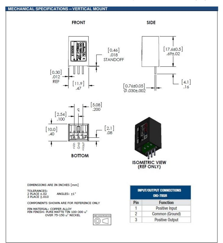
**Encapsulated Non-Isolated Switching Regulator**
