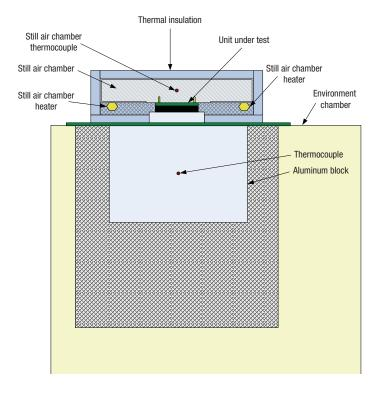
Figure 8. Cold Wall Test Fixture Equipment
