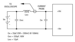
Figure 2. Measuring Input Ripple Current
