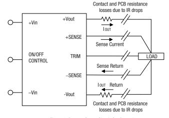
Figure 6. Remote Sense Circuit Configuration
