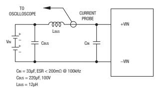
Figure 5. Measuring Input Ripple Current
