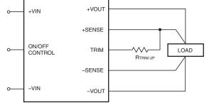
Figure 9. Trim Connections To Increase Output Voltages Using Fixed Resistors
