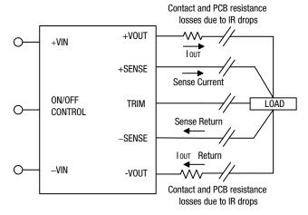
Figure 11. Remote Sense Circuit Configuration
