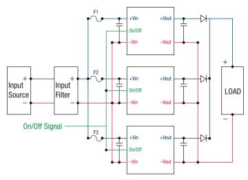
Figure 4. Redundant Parallel Connections
