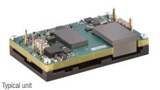
20 Amps) in an industry standard "quarter brick" package requiring no heat sink for most applications. The UWQ series delivers fixed DC output voltages up to 240 Watts (12V @ 20A) for printed circuit board mounting. Wide range inputs of 18 to 60 Volts DC (48 Volts nominal) are ideal for datacom and telecom systems.
