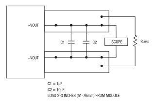
Figure 6. Measuring Output Ripple and Noise (PARD)
