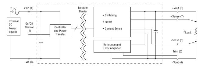
Figure 1. Connection Diagram Typical topology is shown. Murata Power Solutions recommends an external fuse.
