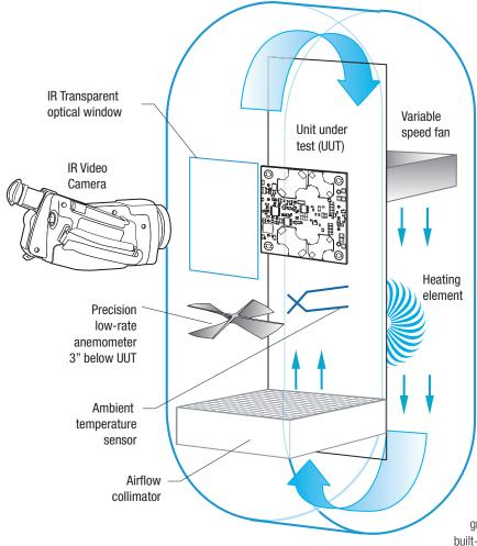
Figure 12. Vertical Wind Tunnel
