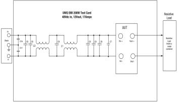
Figure 8. Conducted Emissions Test Circuit
