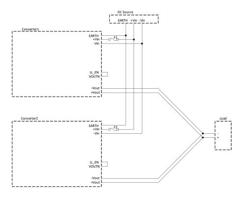
**ORing Feature - Parallel Connection Diagram**
