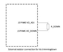
External resistor connection diagram for output voltage adjustment
