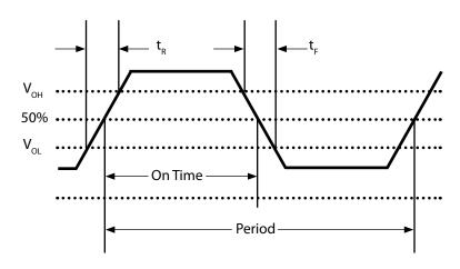
Fig 2: LV-PECL Waveform
