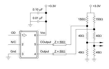
**LV-PECL to LVDS:** Restricted for short transmission lengths. Configuration may require modification depending on LVDS receiver.
