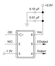
**Production Test:** Allows direct DC coupling into  $50\Omega$  measurement equipment. Must bias the power supplys as shown. Similar to Figure 1.
