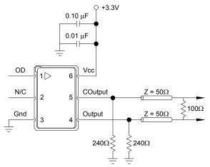
**LV-PECL to LV-PECL:** For short transmission lengths, the power consumption could be reduced by removing the 100 $\Omega$  resistor and doubling the value of the pull down resistors.
