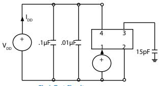
Fig 1: Test Circuit
