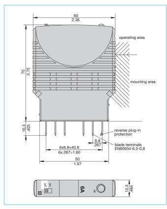
This is a metric design and millimeter dimensions take precedence (  $\frac{mm}{inch})$
