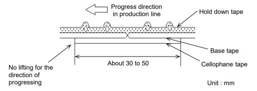
b) When hold down tape is spliced
