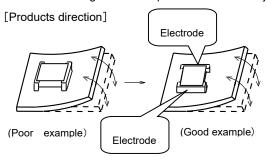
The electorode part of the products should be located like the picture to the mechanical stress.
