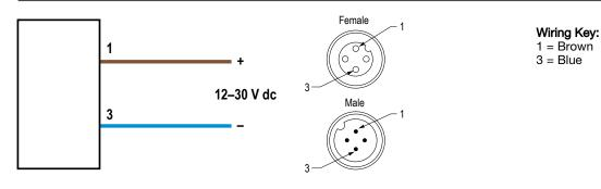
Integral QD models only are listed. For integral 2 m (6.5 ft) PVC cable, omit suffix Q from model number (for example, WLAW105X180E). A model with a QD requires a mating cordset (see *Cordsets* (p. 3)).
