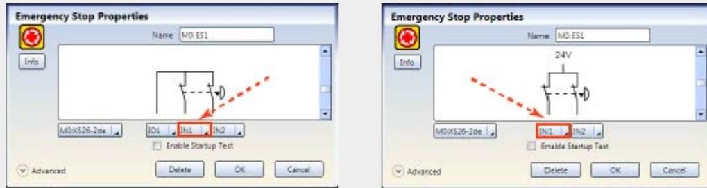
Figure 22. Manually Configured Circuits
