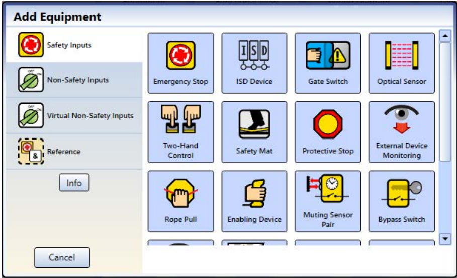
Figure 55. SC10-2: Adding inputs from Equipment View (physical status output can only be added from this view)
