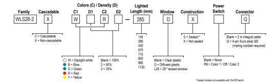
Density (D) is defined by the quantity of LEDs populated on the circuit. For example, at 100% density, there are 18 LEDs per 285 mm, and at 50% density, there are 9 LEDs per 285 mm. The lumen output decreases proportionally with density.
