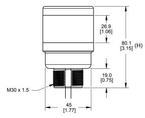
Figure 1. Standard Model Dimensions
