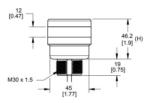
Figure 2. Compact and Beacon Model Dimensions
