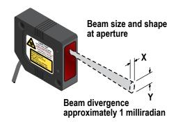
Figure 3. Minimum object detection size vs. distance
