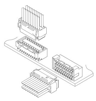
To meet the requirement of the high density mounting on PC board of flat panel TV, AV equipments etc., this connector is designed to the double-row type of 1.25 mm pitch.
