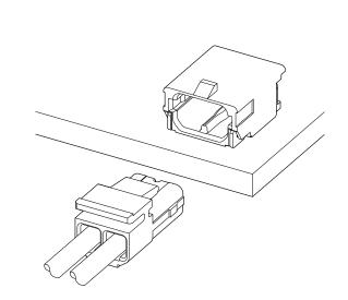
This SFK connector is a wire-to-board connector for connecting power supply and PCB and withstands high voltage. It is used for power supply of LED backlight in Liquid Crystal Display Television set.
