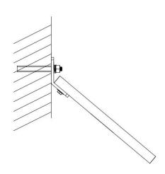
The bracket is fixed at a 40degree tilt which is generally a good tilt for most applications.
