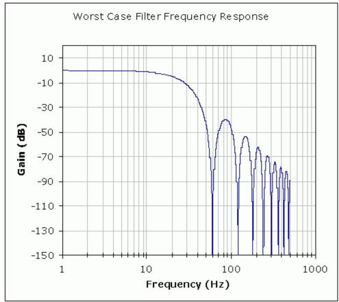
Figure 1. Nominal clock source gives infinite 60Hz rejection.
