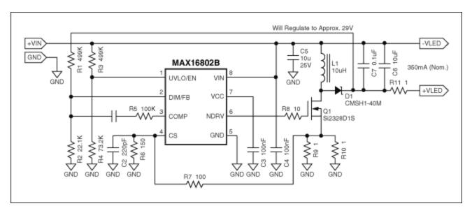
**Caution:** Avoid applying power to the circuit with the  $+V_{LED}$  and  $-V_{LED}$  terminals not connected to an LED.
