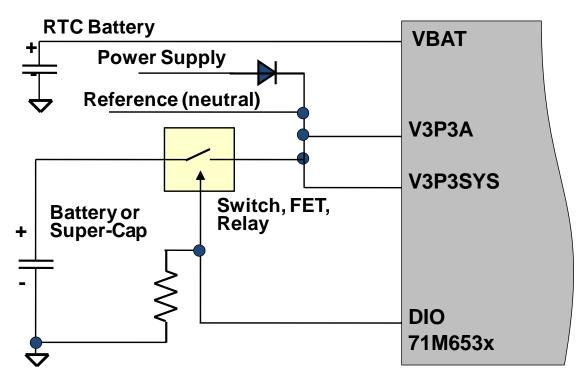
Figure 1: Sample Circuitry for Return to BSMM
