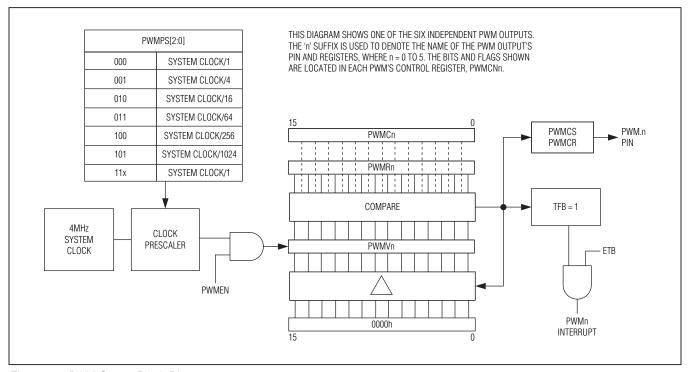
Figure 9-1. PWM Output Block Diagram
