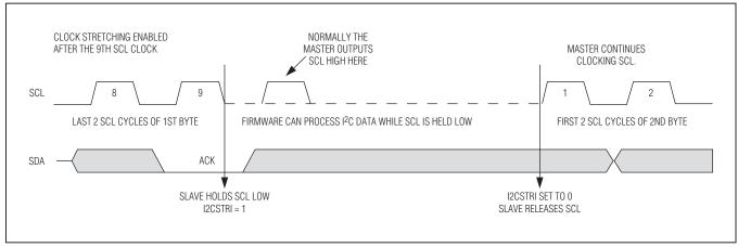
Figure 7-3. Slave I<sup>2</sup>C Clock Stretching
