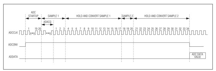
Figure 6-2. Extended Acquisition Time
