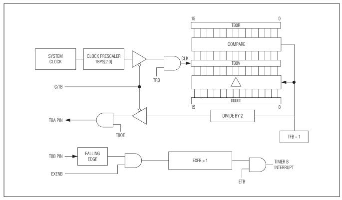
Figure 12-4. Clock Output Mode Block Diagram
