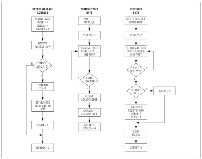
Figure 7-2. Slave I<sup>2</sup>C Data Flow
