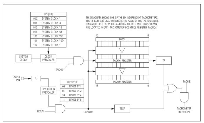
Figure 10-1. Tachometer Input Block Diagram
