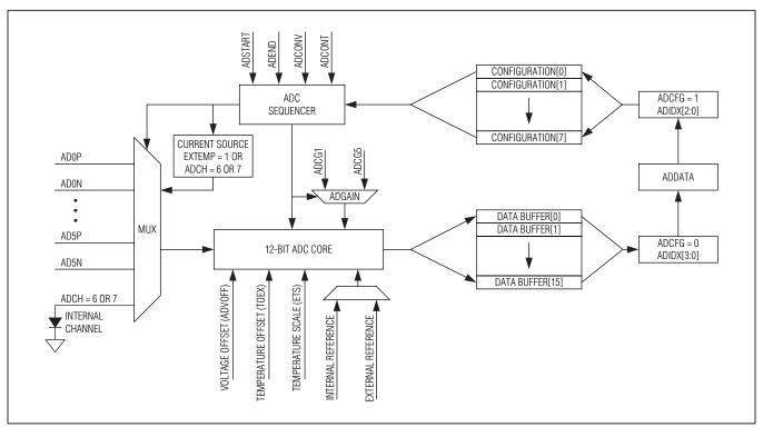
Figure 6-1. ADC Functional Block Diagram
