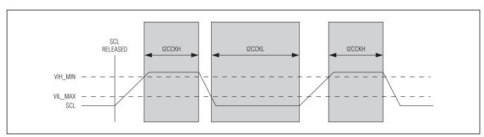
Figure 8-1. I<sup>2</sup>C Clock Generation
