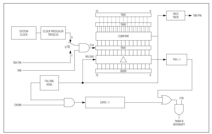
Figure 12-5. PWM Output Mode Block Diagram
