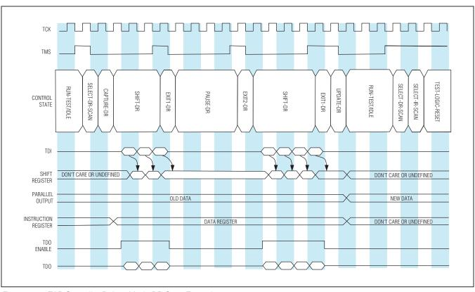
Figure 16-4. TAP Controller Debug Mode DR-Scan Example
