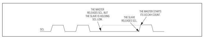
Figure 8-2. Master I<sup>2</sup>C Clock Generation During Slave Clock Stretching
