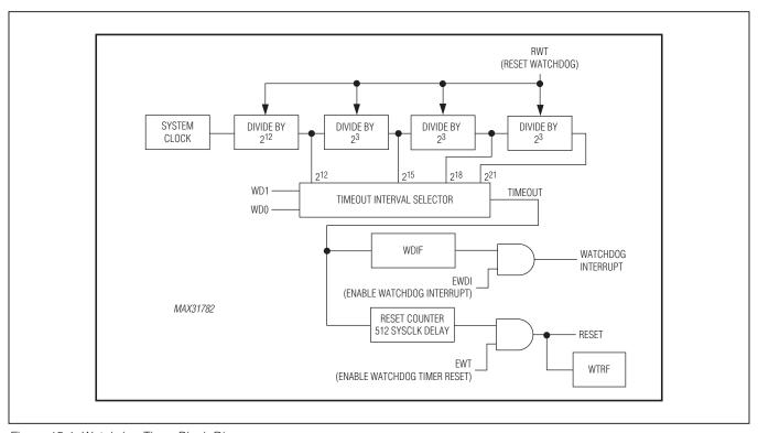
Figure 15-1. Watchdog Timer Block Diagram
