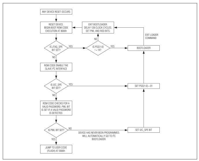
Figure 18-1. Entering Bootloader Operation
