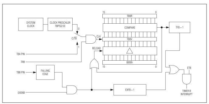
Figure 12-1. Auto-Reload Mode Block Diagram
