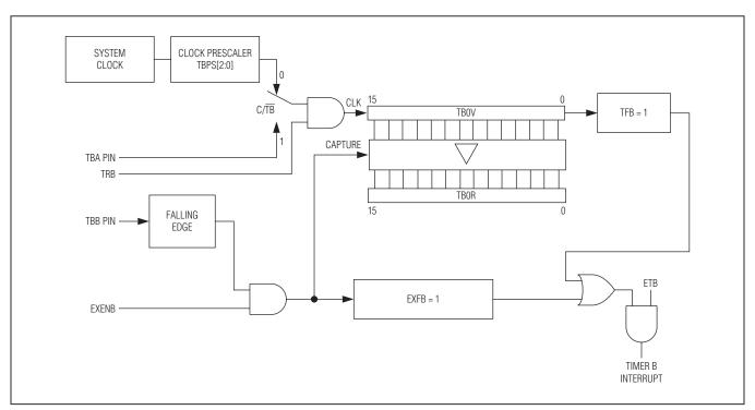
Figure 12-3. Capture Mode Block Diagram
