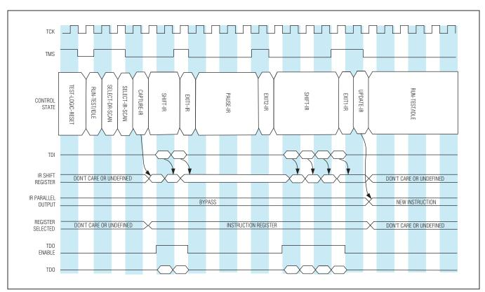
Figure 16-3. TAP Controller Debug Mode IR-Scan Example
