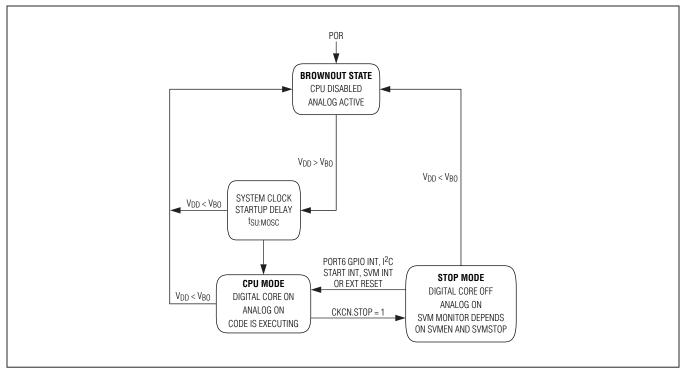
Figure 2-6. MAX31782 State Diagram
