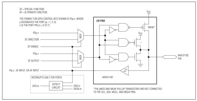
Figure 11-1. GPIO Pin Block Diagram
