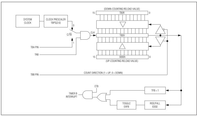
Figure 12-2. Up/Down Count with Auto-Reload Mode Block Diagram
