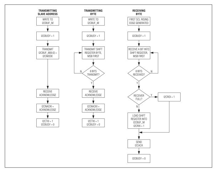
Figure 8-5. Master I<sup>2</sup>C Data Flowchart
