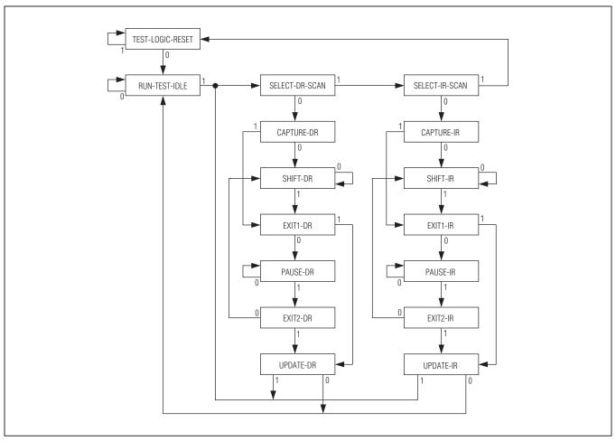
Figure 16-2. TAP Controller State Diagram
