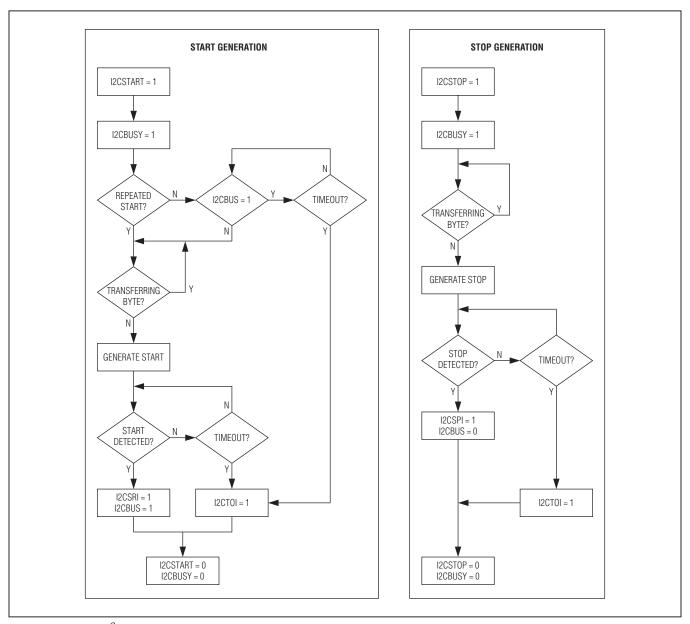
Figure 8-3. Master I<sup>2</sup>C Generated START and STOP
