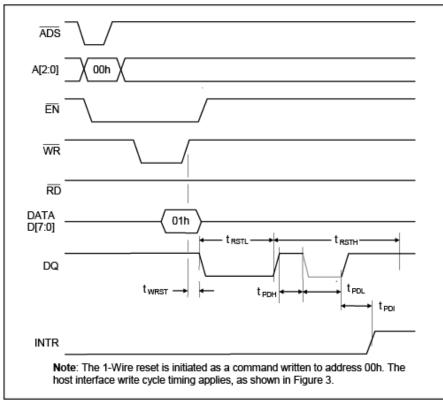
Figure 5. Host interface timing, issuing a 1-Wire Reset.
