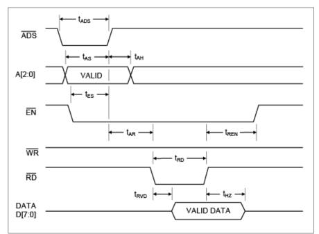
Figure 4. Host interface read cycle.
