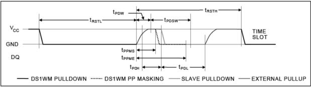
Figure 6. Reset/presence detect cycle.
