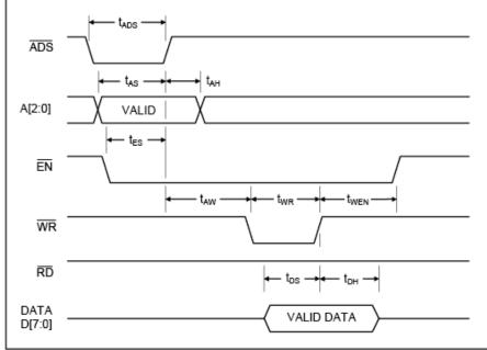
Figure 3. Host interface write cycle.
