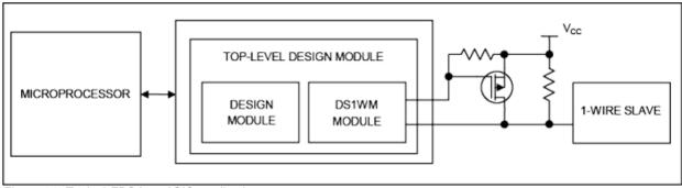
Figure 14. Typical FPGA or ASIC application.
