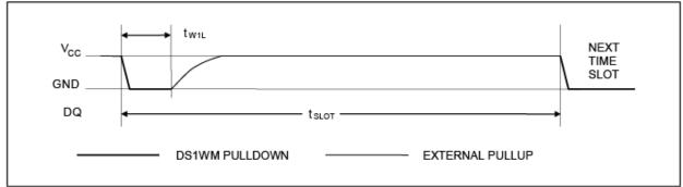
Figure 8. Write-one time slot.
