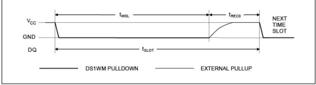
Figure 7. Write-zero time slot.
