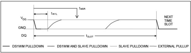
Figure 9. Read-data time slot.
