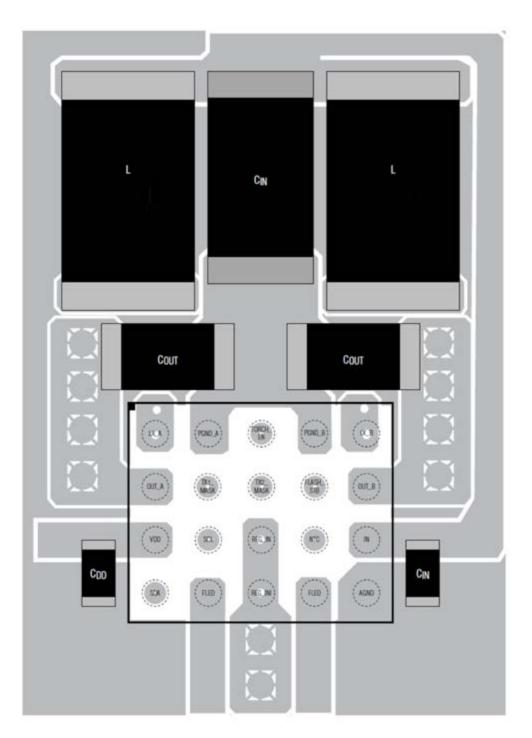
Figure 4. MAX77387 recommended component placement.
