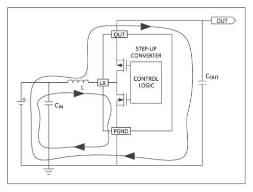
Figure 1. Step-up regulator current loop.
