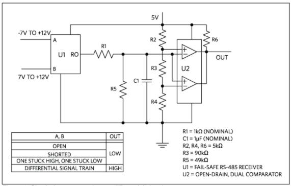
Figure 1. Circuit detects a continuous differential signal.
