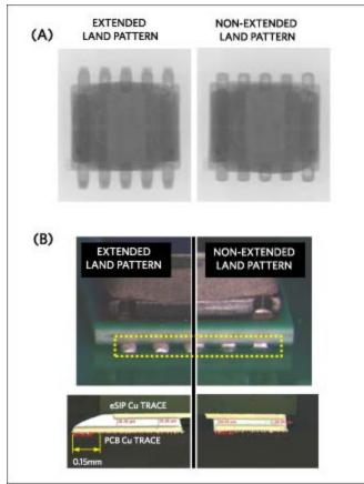
Figure 2. Recommended "extended land pattern" design shows (a) good solder voiding level and (b) is side-inspectable.
