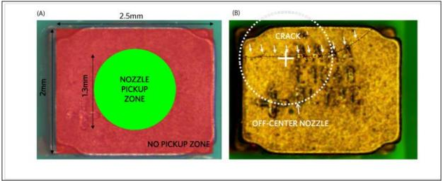
Figure 5. (a) Recommended nozzle pickup region (green circle); (b) inductor top crack could be induced by placing the nozzle outside the pickup zone (example shows using a 1.48mm diameter with the nozzle placed off-center).
