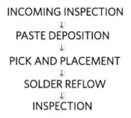
Figure 3. Recommended uSLIC assembly process.
