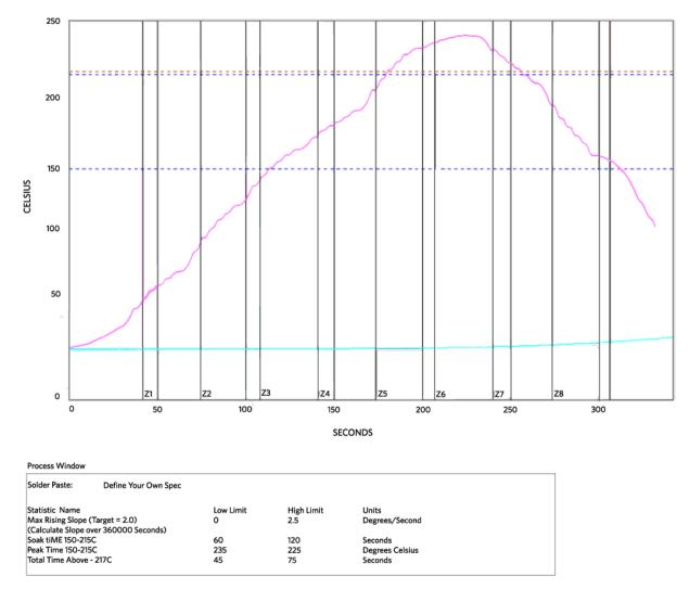
Figure 6. Recommended reflow profile for Pb-free solders per JEDEC JSTD-020.
