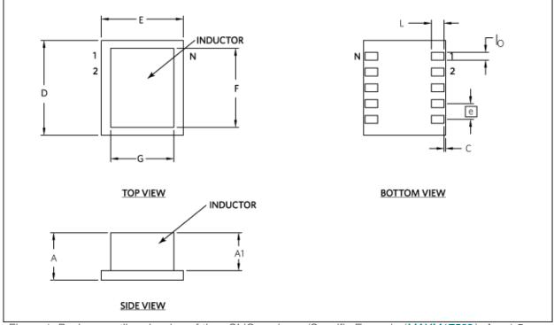
Figure 1. Package outline drawing of the uSLIC package (Specific Example (MAXM17532):  $A = 1.5mm \pm 0.15mm$ , A1 = 1.2mm(max),  $b = 0.25mm \pm 0.05mm$ ,  $c = 0.05mm \pm 0.05mm$ ,  $D = 3.00mm \pm 0.05mm$ ,  $E = 2.60mm \pm 0.05mm$ ,  $e = 0.50mm \pm 0.05mm$ ,  $F = 2.50mm \pm 0.20mm$ ,  $G = 2.00mm \pm 0.20mm$ ,  $L = 0.40mm \pm 0.05mm$ ).
