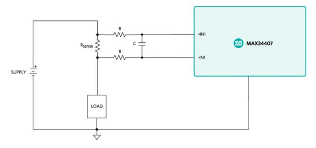
Figure 10. Differential-mode filter.
