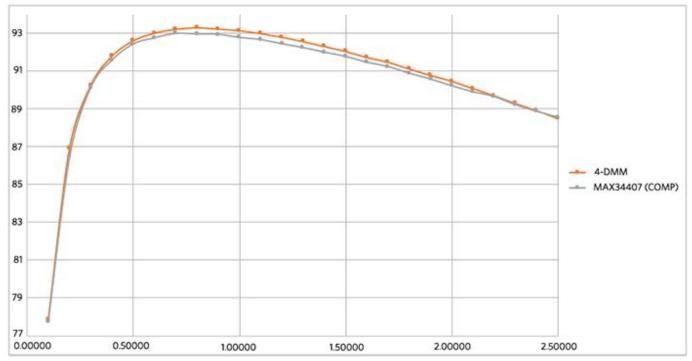
Figure 5. MAX34407 compensated efficiency measurement vs. 4-DMM method.
