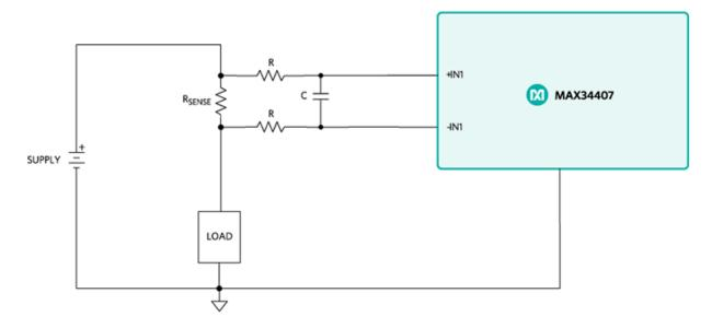
Figure 9. Common-mode filter.
