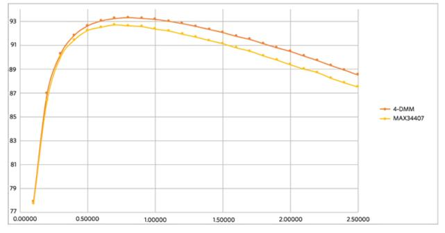
Figure 4. MAX34407 efficiency measurement vs. 4-DMM method.
