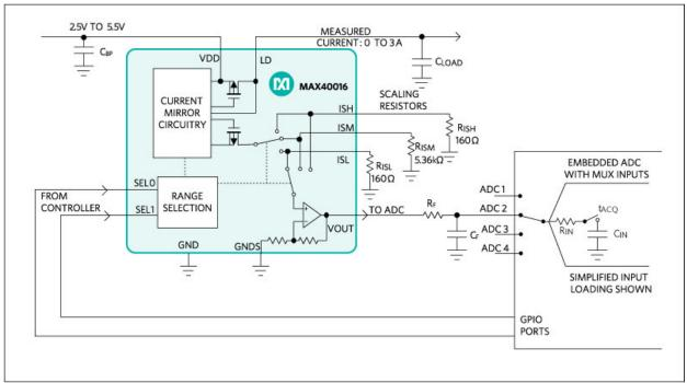
voltage at  $R_{ISM}$  is from 32mV to 1V. For a sense current in the range of 93mA to 3A, the output voltage at  $R_{ISH}$  is from 30mV to 1V.
