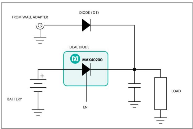
Figure 3. Diode ORing circuit
