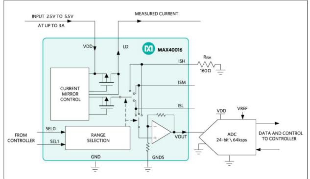
Figure 1. MAX40016 current-sense amplifier with high-resolution ADC to convert output voltage for currentmonitoring.
