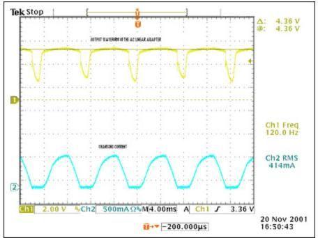
Figure 6. The output waveform of the 3.7V at 350mA AC adapter and the charging current with the MAX1879 charger shown in Figure 5.
