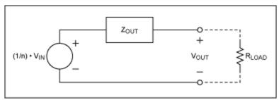
Figure 3. Equivalent circuit diagram of the linear transformer adapter.
