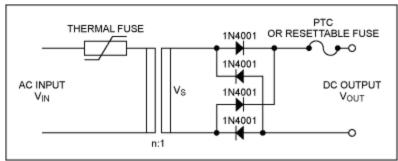
Figure 2. AC linear transformer adapter block diagram.
