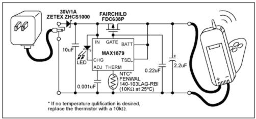
Figure 5. The MAX1879 high efficient Li+ charger.
