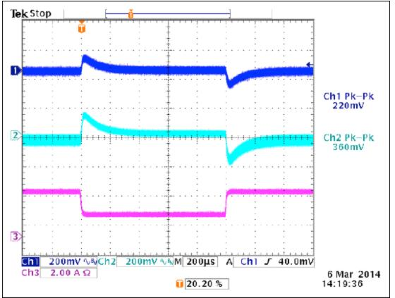
Figure 9. Load step at 5V (100%, 50%, 100% of 3A), 40V input, 3.3V at 0A. CH1: 3.3V rail, CH2: 5V rail, CH3: 5V rail current.
