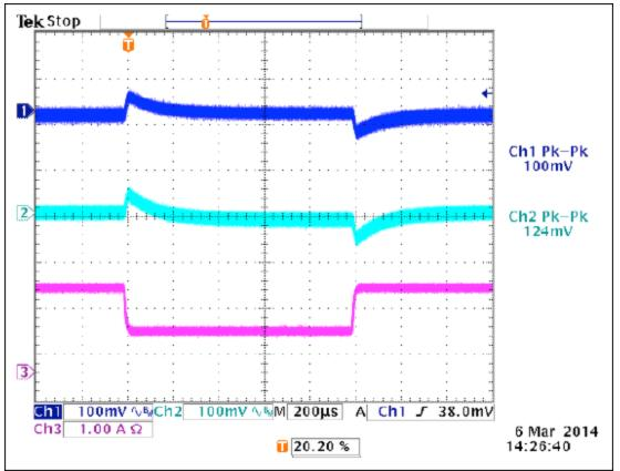
Figure 7. Load step at 3.3V (100%, 50%, 100% of 1.8A), 57V input, 5V at 0A. CH1: 3.3V rail, CH2: 5V rail, CH3: 3.3V rail current.
