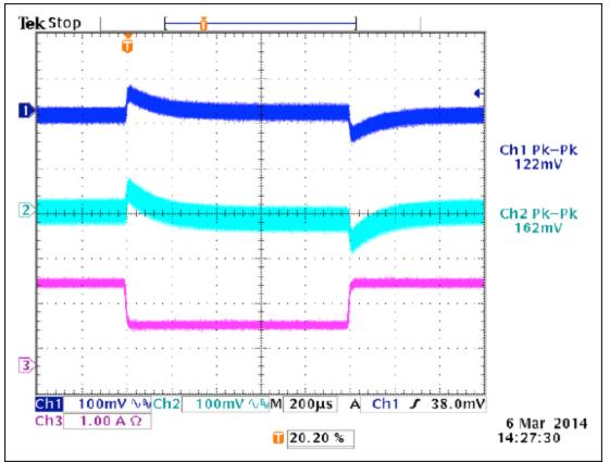
Figure 8. Load step at 3.3V (100%, 50%, 100% of 1.8A), 57V input, 5V at 3A. CH1: 3.3V rail, CH2: 5V rail, CH3: 3.3V rail current.
