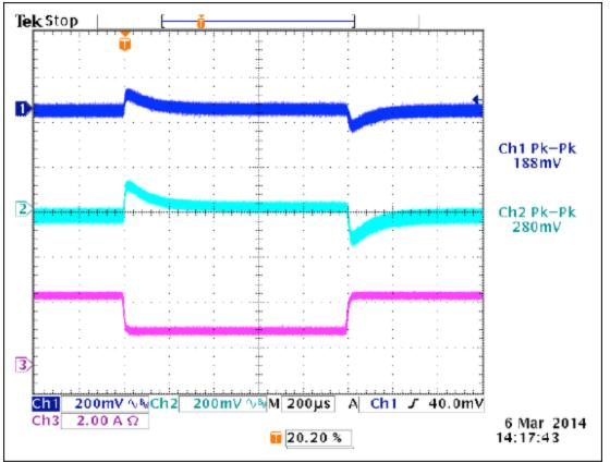
Figure 13. Load step at 5V (100%, 50%, 100% of 3A), 57V input, 3.3V at 0A. CH1: 3.3V rail, CH2: 5V rail, CH3: 5V rail current.
