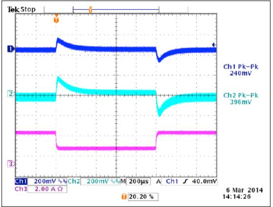
Figure 10. Load step at 5V (100%, 50%, 100% of 3A), 40V input, 3.3V at 1.8A. CH1: 3.3V rail, CH2: 5V rail, CH3: 5V rail current.
