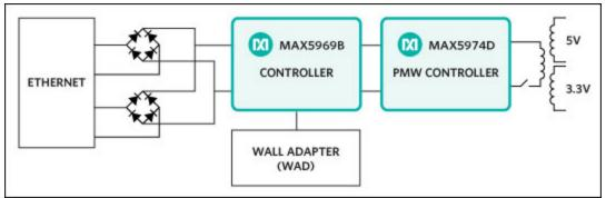
Figure 1. The Pasadena subsystem design block diagram.
