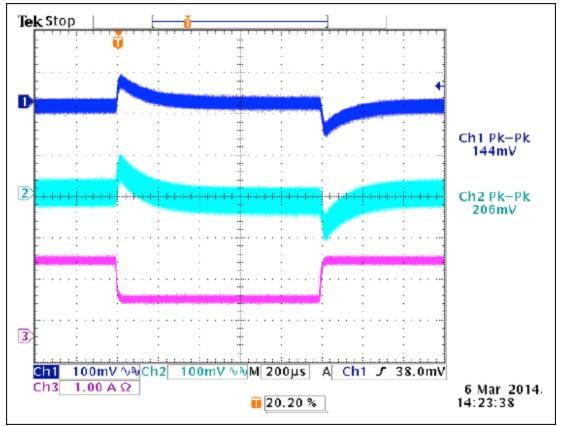
Figure 3. Load step at 3.3V (100%, 50%, 100% of 1.8A), 40V input, 5V at 0A. CH1: 3.3V rail, CH2: 5V rail, CH3: 3.3V rail current.
