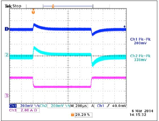
Figure 12. Load step at 5V (100%, 50%, 100% of 3A), 48V input, 3.3V at 1.8A. CH1: 3.3V rail, CH2: 5V rail, CH3: 5V rail current.
