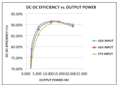
Figure 2. DC-DC efficiency of the Pasadena design, following the diode bridges.
