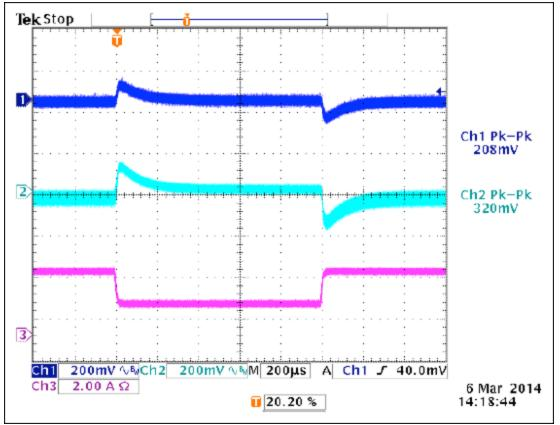
Figure 11. Load step at 5V (100%, 50%, 100% of 3A), 48V input, 3.3V at 0A. CH1: 3.3V rail, CH2: 5V rail, CH3: 5V rail current.
