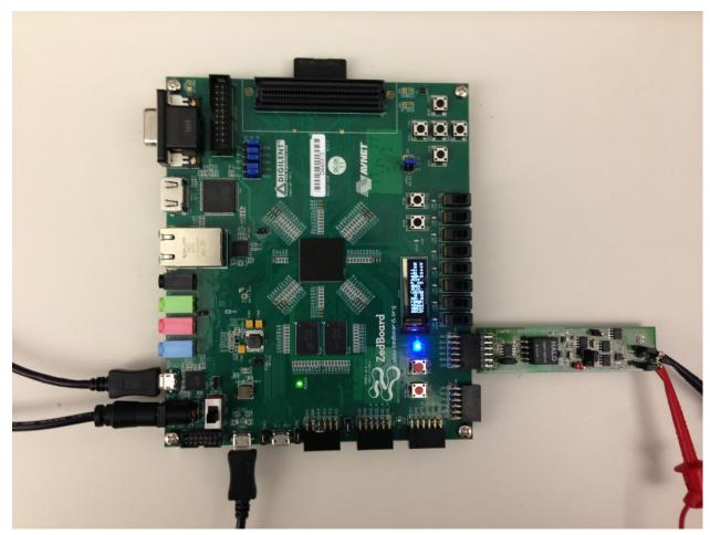
Figure 1. Campbell Board Connected to ZedBoard Kit
