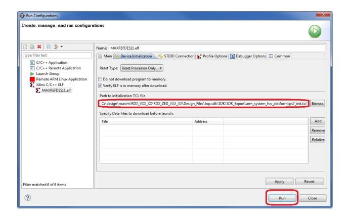
Once the Debug/MAXREFDES4 configuration is set up once, you just need to press the **Run** button if you ever want to run the program again.
