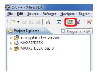
The **Program FPGA** dialog box appears. From here, an FPGA bitstream (.BIT) file is selected. Be sure to select the .BIT file by using the paths below.
