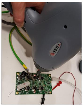
Figure 29. ESD Testing of MAX14819
