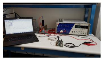
Figure 28. EFT Burst and Surge Testing of MAX14819
