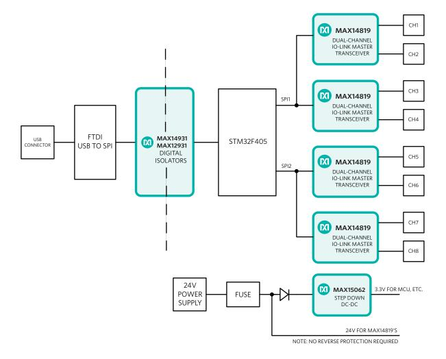
Figure 24. MAXREFDES145 8-Port IO-Link Master Block Diagram
