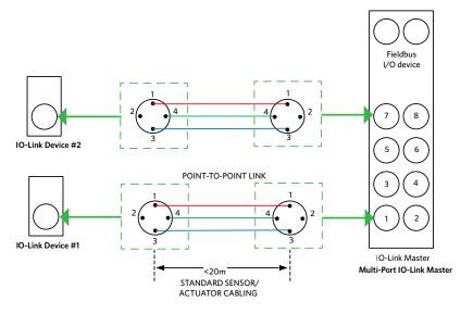
Figure 3. IO-Link Master/Device Interface
