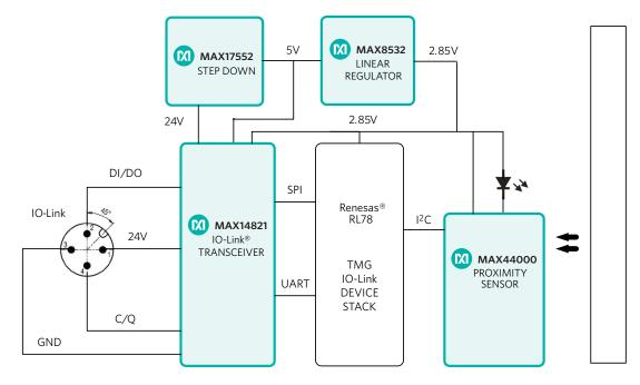
Figure 19. MAXREFDES27 IO-Link Proximity Sensor Block Diagram
