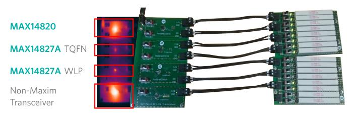
Figure 27. Comparison of Transceiver Power Dissipation at Full Load, Relative to Competitive Device
