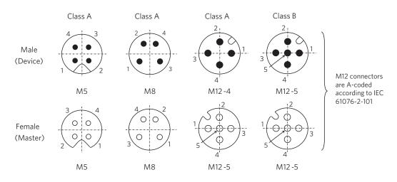
Figure 7. Alternative IO-Link Connectors
