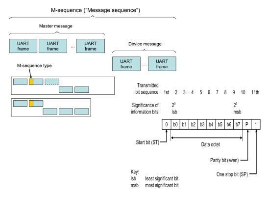
Figure 12. IO-Link Master-Device Communication Sequence
