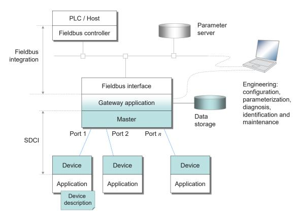
Figure 9. IO-Link Fieldbus Interconnection
