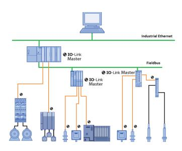
Figure 5. IO-Link Compatibility with Existing Industry Protocols
