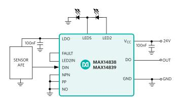
Figure 2. 24V Pin-Configurable Industrial Sensor Output Driver
