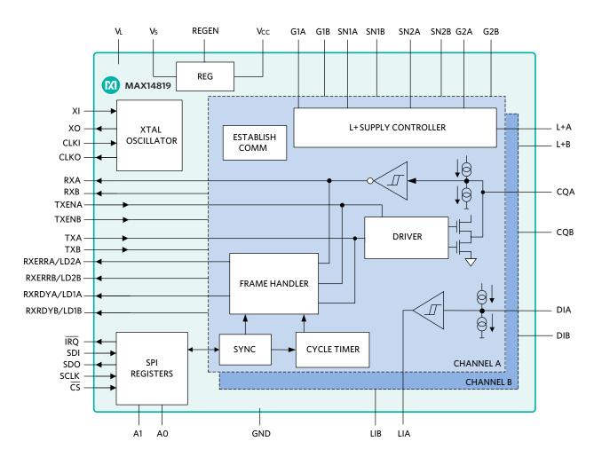
Figure 33. MAX14819 Dual IO-Link Master Transceiver
