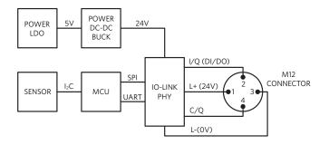
Figure 17. Building Blocks of an IO-Link Sensor
