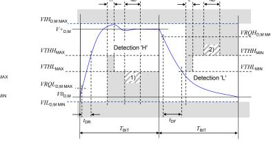
NOTE In the figure, 1) = no detection 'L'; and 2) = no detection 'H' Figure 8b. IO-Link Signal Electrical Characteristics
