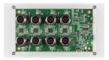
Figure 23. MAXREFDES145 8-Port IO-Link Master Reference Design
