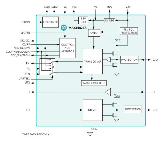
Figure 32. MAX14827A Dual-Channel IO-Link Transceiver
