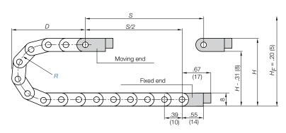
Supplement part number with required radius. Example: 03-05-028-0 Pitch: .39 in. (10 mm) per link links/ft (m) = 30.47 (100)
