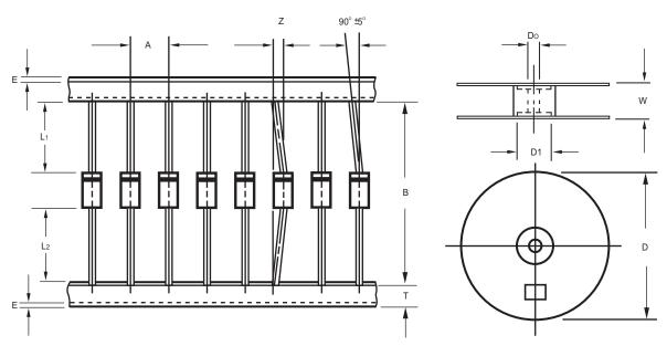
Fig.: Configuration of AXIAL LEAD TAPING
