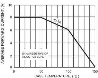
FIG. 2 - TYPICAL FORWARD CURRENT DERATING CURVE
