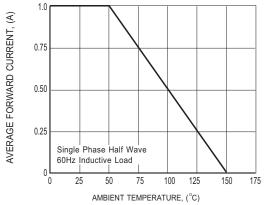
FIG.1 TYPICAL FORWARD CURRENT DERATING CURVE
