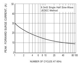
FIG.4 MAXIMUM NON-REPETITIVE FORWARD SURGE CURRENT
