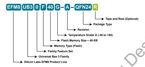
Figure 2.1. EFM8UB3 Part Numbering
