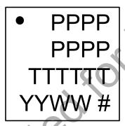
Figure 9.3. QFN20 Package Marking
