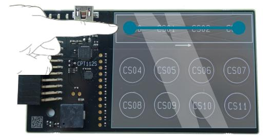
2. Place a finger on any one of the buttons: CS04, CS05, ... , CS10.
