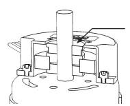
Encoder Cross Section - note the top face of the filler hub should be slightly below the top face of the encoder housing as shown by the arrow pointer.
