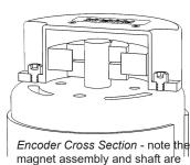
Encoder Cross Section - note to magnet assembly and shaft are not in contact with the encoder housing or the motor housing.
