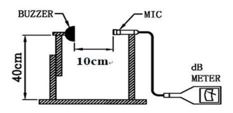
Mic: RION S.P.L meter UC30 or equivalent S.G: Hewlett Packard 33120A Function Generator or equivalent
