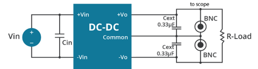
Figure 3 Measuring Output Ripple & Noise for Dual Output Models
