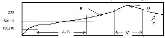
A: Preheating Time:  $60 \sim 120$  Sec. B: Preheating temp:  $150 \pm 10$  °C.
