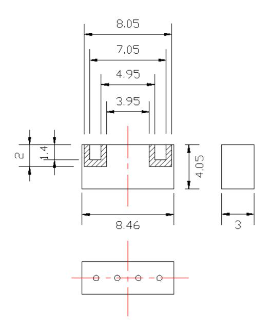
Dimensions in mm Tolerance:±0.25
